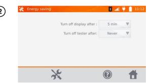
Set the inactivity time for blanking the screen and turning off the meter.
