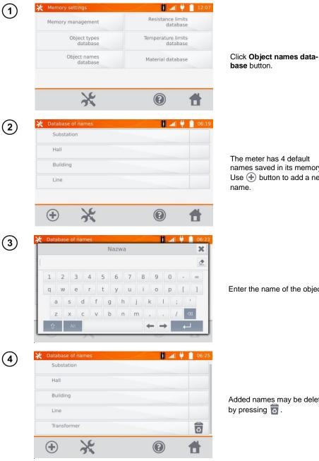
The meter has 4 default names saved in its memory. Use 🕀 button to add a new
